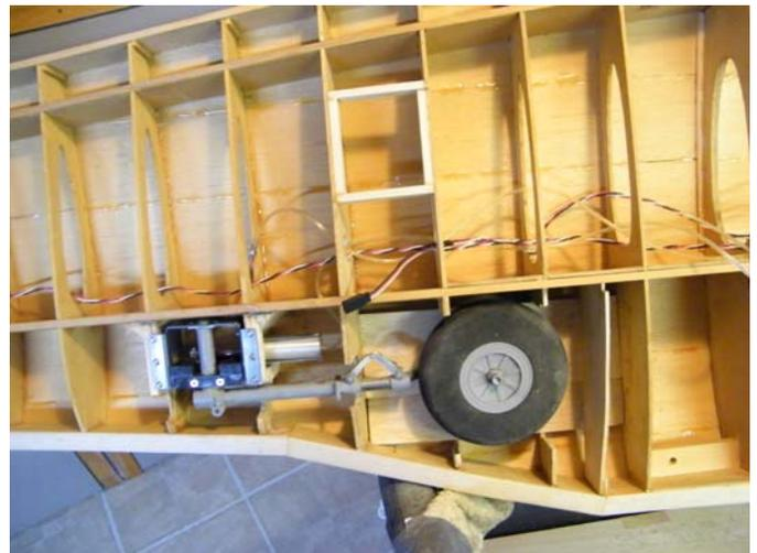
servos in the bays where the bellcranks should be and now I need to sheet the bottom of the wings and glue and shape the wing tip blocks in place to complete the wings. Oh! And the Flaps which are enormous and the Ailerons are hinged with hinge points and fitted. Same set up for the Elevators and Rudder
