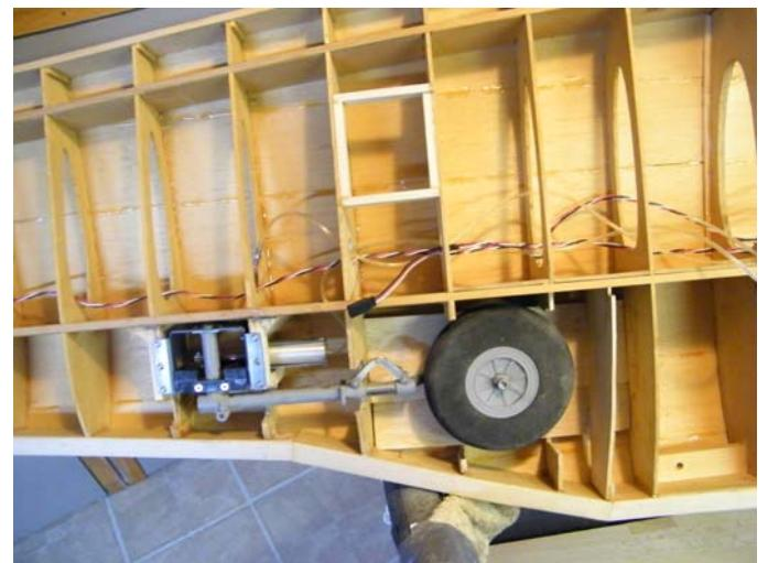
servos in the bays where the bellcranks should be and now I need to sheet the bottom of the wings and glue and shape the wing tip blocks in place to complete the wings. Oh! And the Flaps which are enormous and the Aelerons are hinged with hinge points and fitted. Same set up for the Elevators and Rudder
