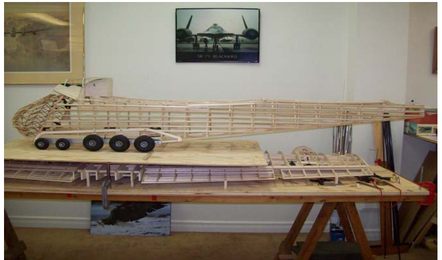
Fuselage for both Me 321 and Me 323 versions
