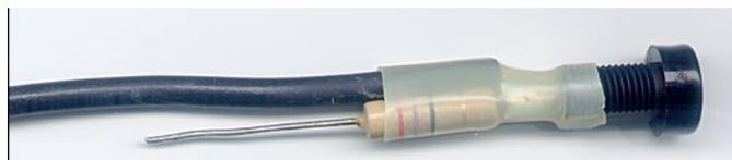
Bend up and solder the other lead of the resistor to the red banana jack. Also solder on the red wire.
