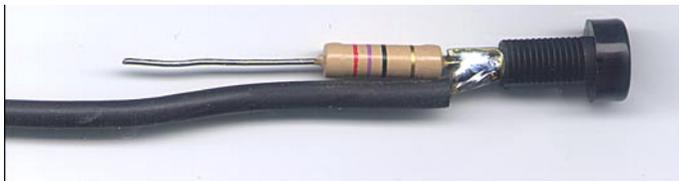
Cover the resistor and connection with heat shrink tubing or electrical tape.
