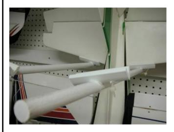
I then cut 3" lengths of corner molding made out of this same composite material (saves painting). You need two for each plane. This is great because you don't need any foam and the weight is spread over 6" (no bruising on your stab leading edge!).
