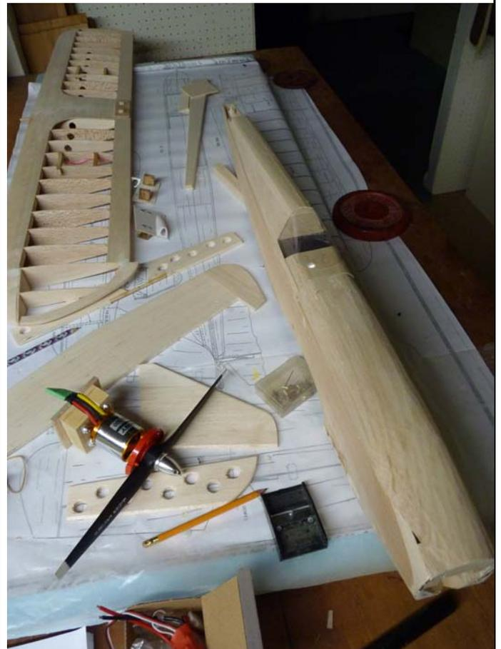
my waste bin. There is a lot of wood in this kit and most of it gets itself into shavings it seems. I built the "power module" in one and this slides vertically into the fuselage. I had yet to figure out what stops it sliding vertically out however.
