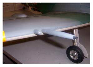
tip over landing. Knowing this I decided to build in some sacrificial break off points that would make repairs a simple process of just adding a dab of CA to the base nut. I used 5/16th dowel turned down on my bench drill press, added a short tube for the cannon barrel and then a small screw and nut to finish of the effort. Paul Chitty liked these so much I made him a pair for his Spitfire too. The gun camera lens is a simple cupboard door
