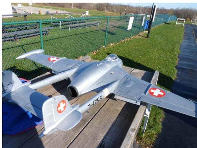
12 bladed EDF with a very aggressive pitch and balanced by Eric. The fan is powered by a 1600kva motor. Fuel is a 6s, 5500 mah li-po. I saw this aircraft take off in about 10 feet in a 5 Knot headwind. The EDF sounds more like a Gas Turbine than...well most gas turbines and the balanced relatively low speed fan is smoooooth as silk. Ted Pritlove now has one of these too so we can look forward to some formation flying. Right Ted?
