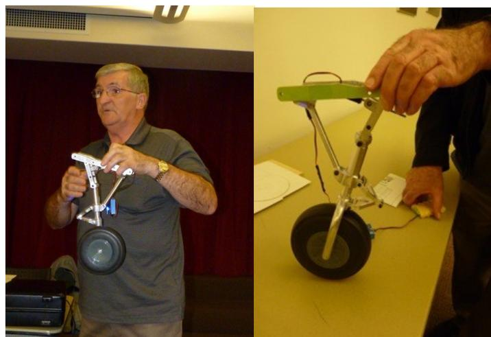
Karl Gross showed us the landing gear for the Cessna Crane he has been working on. Above is the mock-up Karl used to make sure it worked—a few adjustments were needed after which he machined the gear!
