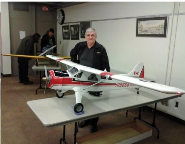
Karl Gross’ latest addition to his fleet is a red and white Dehavilland Beaver from Hangar 9. This ARF kit is a little under .25 scale, weighs in at 17 lbs. and is powered by a Saito 180. The landing and navigation lights which are not a part of the kit are from Electro Dynamic. Karl is very impressed with the quality of the kit and said that the only problem is that the fuel tank that comes with the kit is not appropriate and needed some MacGyvering, a concept that is not new to Karl
