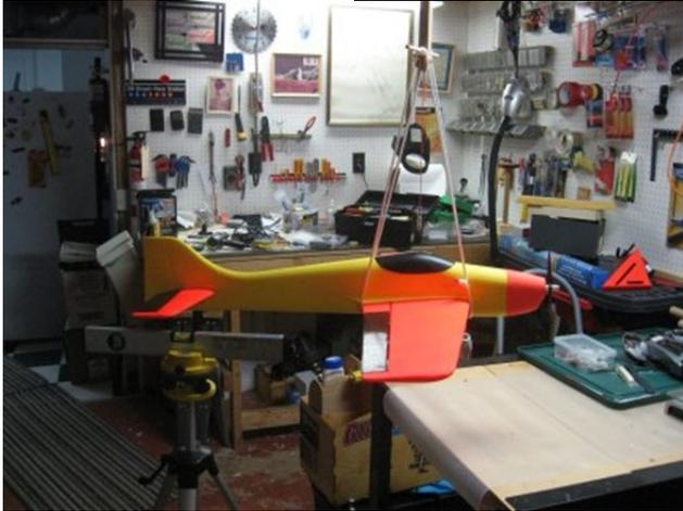
Joe Fazzari demonstrated the design and use of the Vanessa CG Machine which he uses to balance his aircraft. He stated that although the device took only 15 minutes to manufacture out of scrap found in his workshop, it took him 2 weeks to figure out how to work it due to the fact that there is no article or video on the internet that does a good job of tying all aspects of the device together.
