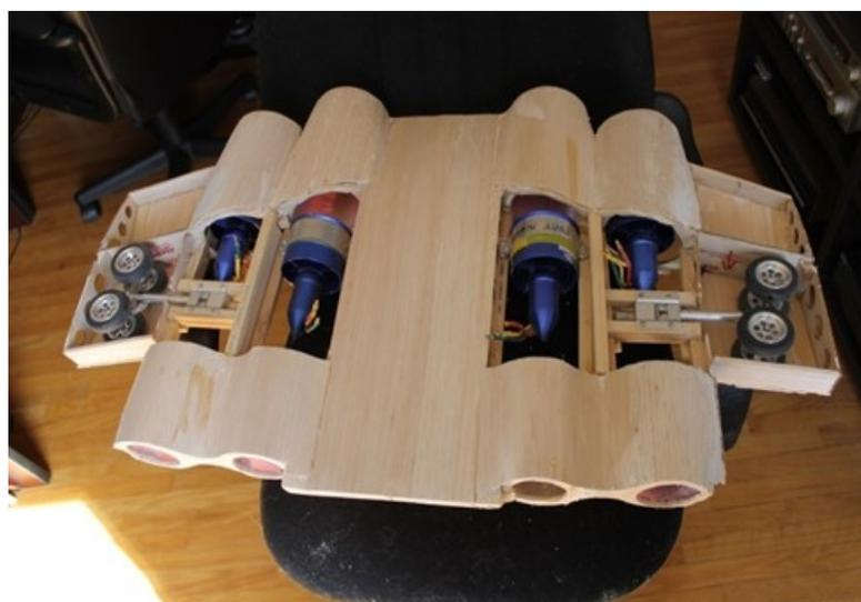
I decided on Nav and Landing lights so it has 2mm LED landing lights in each wing and red and green wing tip, white tail and upper and lower red rotating beacons all driven from a separate Lipo pack. All of the electronics, EDF's, undercarriage and batteries are from Hobby King. All that remains to be done at this time is the finish sanding and fibre glassing.
