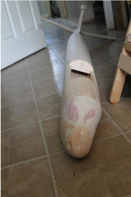
So at this time the major airframe work is done, I now need to finish and fibre glass the whole thing, install the tail servos and nose wheel steering servo and find a safe home for the 10 channel receiver.
